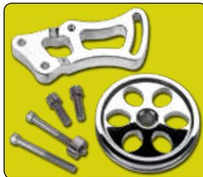
Machined billet aluminum bracket bolts to the front of the engine block with the two bolts next to the timing chain cover. Supplied V-belt pulley must be used for proper alignment. 3 groove crank pulleys required in all applications. Professionally polished.
