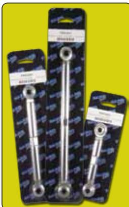
Polished aluminum adjuster bars complete with zinc finish steel left and right heim ends for 3/8" bolts. Bar is 5/8" diameter and features square milled into it for a wrench to fit while you tighten the jam nuts. With ends threaded all the way in the center to center measurements are about 1/8" shorter than listed lengths and can be extended out about 1" safely.
