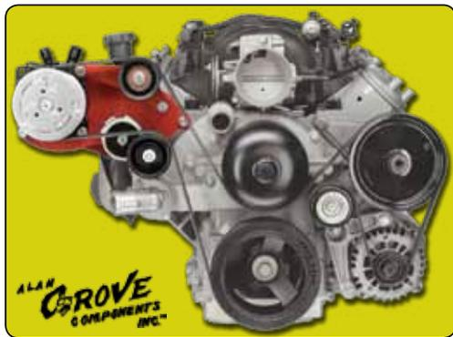
This bracket system is designed to mount an aftermarket Sanden 508 compressor to the popular LS series engines utilizing the factory alternator and power steering pump accessories. Bolts to head and water pump. Works well in vehicles with low hood clearance - Trucks, 50-60's cars, etc.
