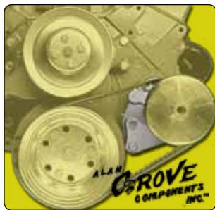
Steel bracket sits the pump high enough to clear most chassis parts and steering gears. Bracket bolts off the front of the engine block only. Requires 3 groove crank pulley in all applications. Will work with power steering pumps with attached composite reservoir. Aluminum pulley fits 17mm pump shaft that is a press-on style.
